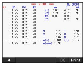
When the measurement is made with the IOL measurement mode, `I' is indicated on the left side of the measurement value.
