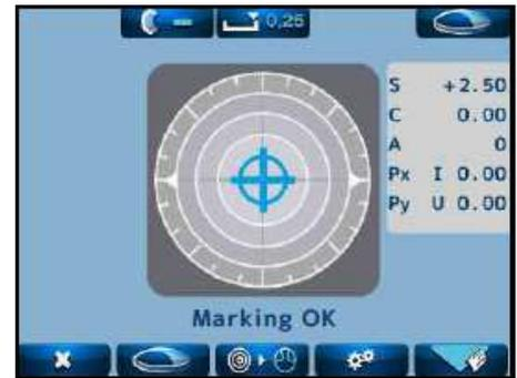
(3) Take a measurement of near point after confirming that “Ad1” is displayed. Move the lens so as that the near point (near-sight segment) comes to the center of the lens stand.
