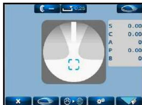
In case that **Auto Prog** is set as “**On**”, the lens is automatically judged whether the lens is a progressive lens or not.
