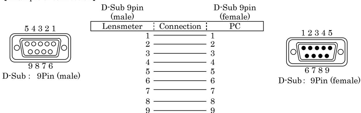
Use the straight cable (D-sub 9 pin: male/ D-sub 9: female) as the connection cable at the time of outputting the measurement values by using the RS232C.
