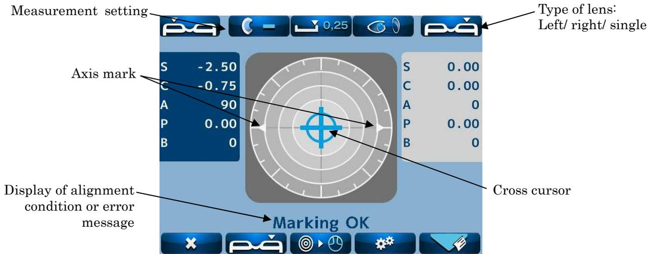
Measurement screen of single focus lens, multifocal lens and contact lens
