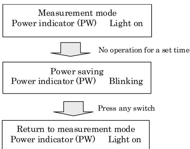
While this function is activated, the power to the measurement light and LCD monitor is turned off. It returns to the measurement mode by pressing any switch.
