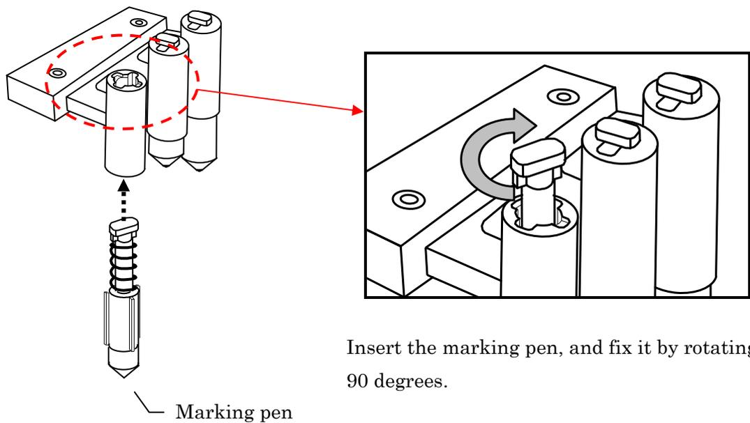
Insert the marking pen, and fix it by rotating 90 degrees.
