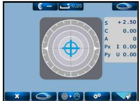
※ In case of setting "**Auto Memory**" on the Setup screen as "On", the measurement values are stored in memory automatically after the message "Marking OK" appears.
