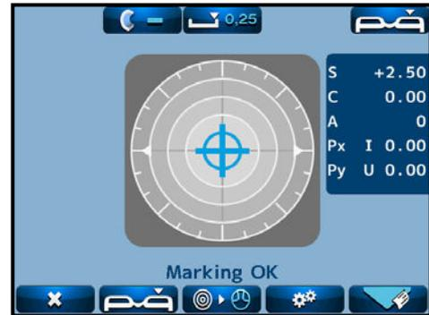
(4) Save the measurement values in memory by pressing the Memory/Add switch after measurement. The color of the measurement value area is changed, and the measurement values are fixed.
