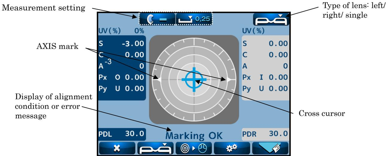
Measurement screen of single focus lens, multifocal lens and contact lens
