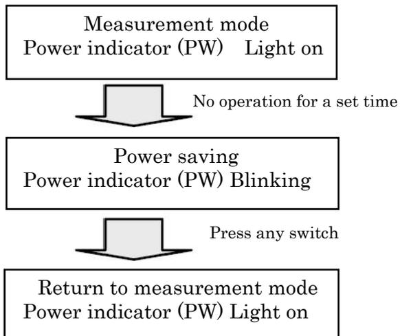
While this function is activated, the power to the measurement light and LCD monitor is turned off.
