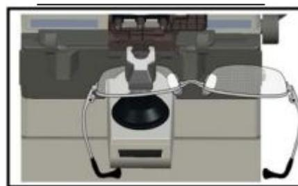
➤ Read the power by setting the cross on the center for Single vision lenses , or in the square for progressive lenses.
