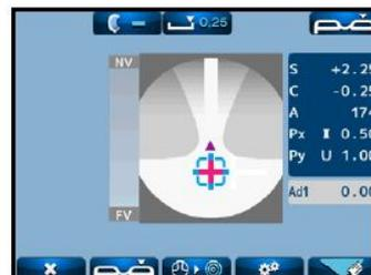
Read left lens by moving the frame to the right
