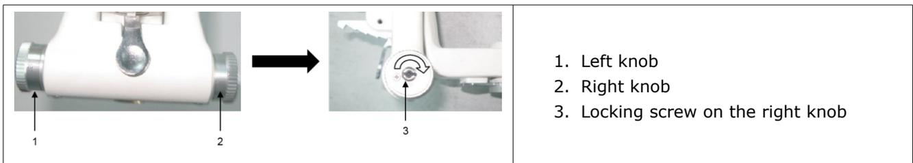
2 Rotate the locking screw with a hexagon type screw driver.
