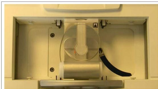
9. Then place the pattern holder in the tracing chamber (see Chapter 4, Special cycles: pattern tracing),
