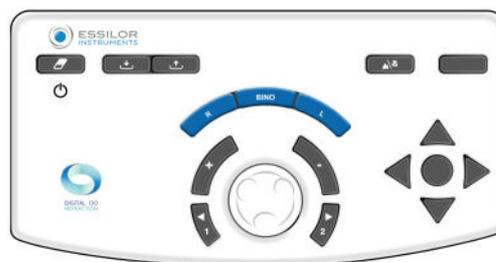
2 Turn the console keyboard's central button clockwise (-) or counterclockwise (+).
