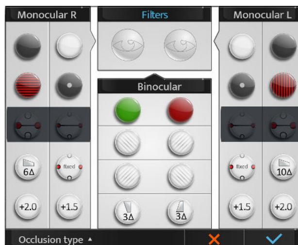
Press on [Occlusion type] and select the desired type of occlusion from the list:
