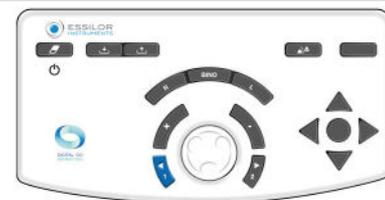
To show the dots in position 2, press, press the "2" key on the console keyboard.
