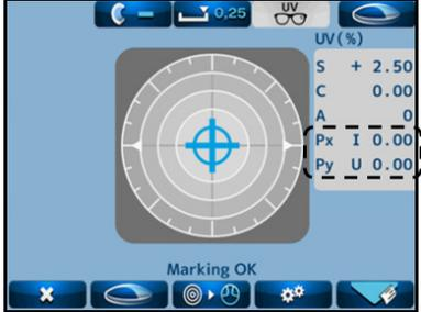
Furthermore, [Prism Center] on the Setup screen set to [On], It is possible to enter any prism center value on the following screen.
