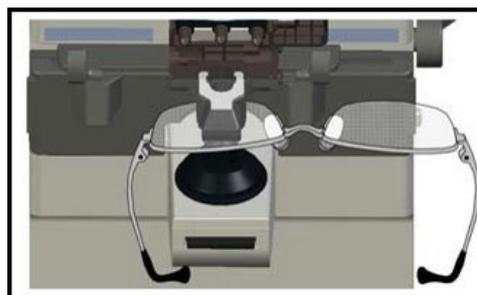
At this time, it is switched from right lens to left lens automatically based on the position of the nose pad.
