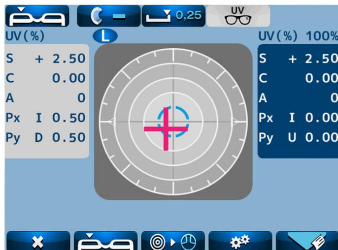
In case of measuring PD with the setting of PD Measure [On], the right eye and left eye are switched automatically.
