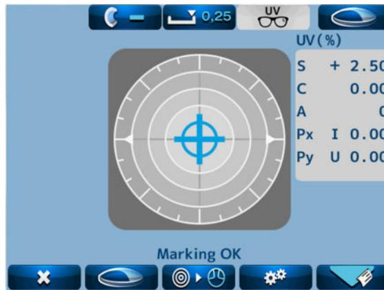
In case of setting [Auto Memory] on the Setup screen as [On], the measurement values are stored in memory automatically after the message [Marking OK] appears.
