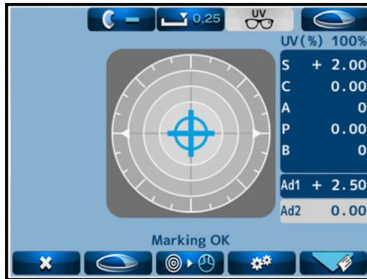
In case of trifocal lens, display "Ad2" by pressing the Memory/Add switch one more time. After that, repeat (3) and (4) after bringing the second near point (near-sight segment) to the center of the lens stand.
