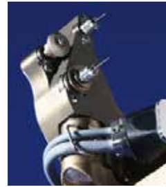
Integrated module with 3 removable spindles: Groove-Milling, High Curve-Chamfer and Drilling
